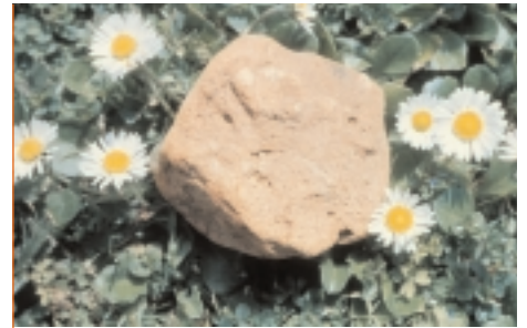
A piece of Roman brick from the Theatre at Fiesole, near Florence, Italy. Although this fragment is about 2000 years old it is similar in composition and texture to Australian bricks of the 18th century.
